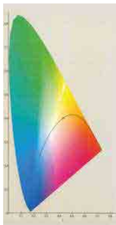
Spectral distribution (left) and color coordinates show that our DLED4 bicolor light (in tungsten function) is perfectly placed on the Planck Curve (right).
